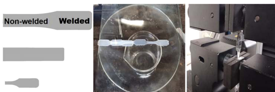
Figure 2. Representation of PP dog bone specimens and their area locations used for mechanical property calculations as given in Table 1 (left), digital images of both the experimental setup (middle), and the welded small dog bone sample fixed between clamps (right).
